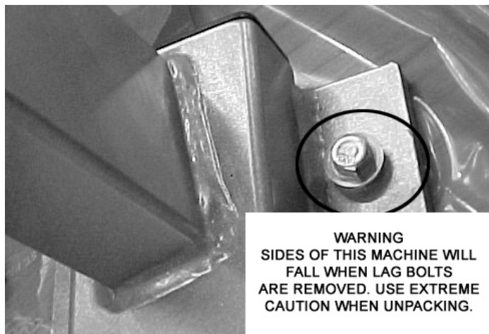
Unpacking Figure 2. Lag shipping bolts.
